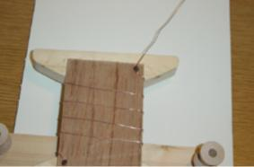
Drive two small tacks part way into opposite corners of the spool base so they will also go into the end pieces, wrap one end of the wire around it and drive it in all the way. Loop the wire around the spool base in a spiral so you end up at the other end, wrap the wire around the other tack, trim the end and drive the tack all the way in.
