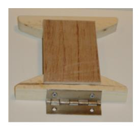
When the hinge is attached lay it on the base in the same manner and center the hinge on the base with the holes in the screw 1 1/2" from the back edge. Fasten the hinge to the base with 5/8 X 6 wood screws.
